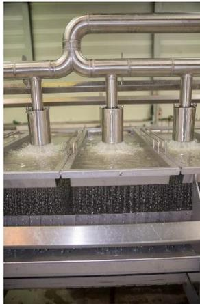
The OctoFrost™ IF Chiller has been designed to exceed all international regulations on food safety and hygiene. Every part of the chiller which comes in contact with the chilling water can be cleaned by CIP (Cleaning-In-Place).
