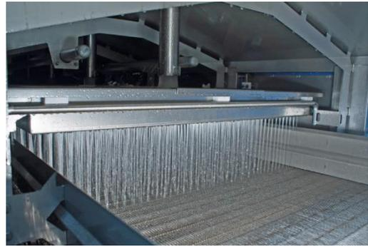
Water consumption is only caused by water pick-up on the product which usually ranges between 5% and 10% of the production capacity (e.g. for a 2000 kg/h production, water consumption would amount 140 l per hour).
