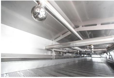
All piping, Aisi 316 stainless steel, is *backing-gas* welded. This method ensures the highest hygienic standard possible.
