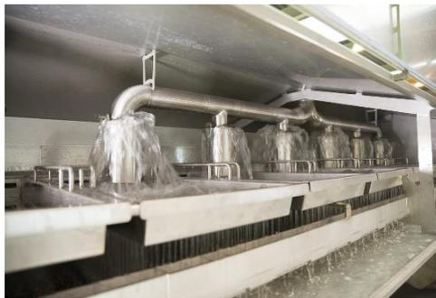
The water in the OctoFrost™ IF Cooker is heated by means of direct steam injection, which is absorbed completely into the water. A high volume of recirculated water is used which has a very low temperature-drop when exiting the cooker ( $\Delta T$  - max. 3° C), therefore very little steam is needed to reheat the water translating in
